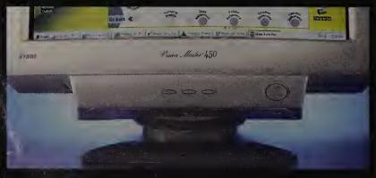
IIYAMA USES FEWER BUTTONS: You access most of the individual controls by using the on-screen display's menu system.
